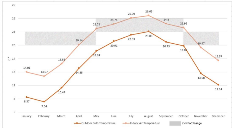
Figure 48: Effect of Using Low Energy Triple Glass with 3.81 cm Thick Expanded Polystyrene to East oriented Scenario
