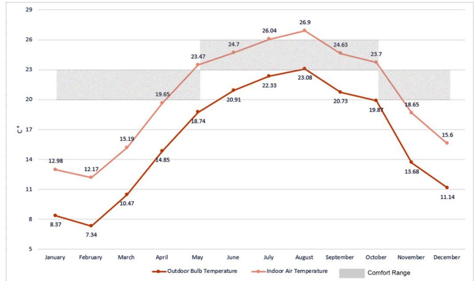
Figure 43: East Oriented Scenario – Building Thermal Performance
