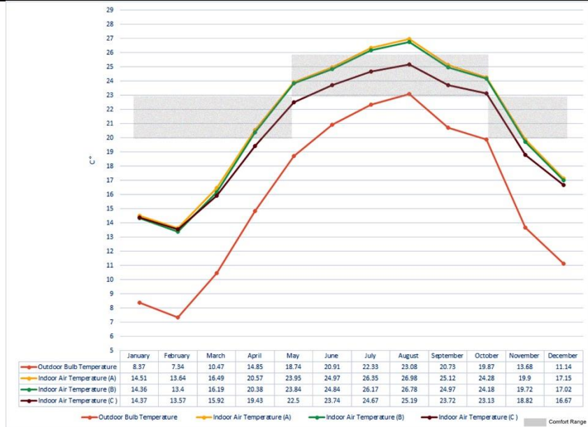
Figure 66: East vs. West Envelope at Roof Level vs. East Envelope at Ground Floor Level – Building Thermal Performance
