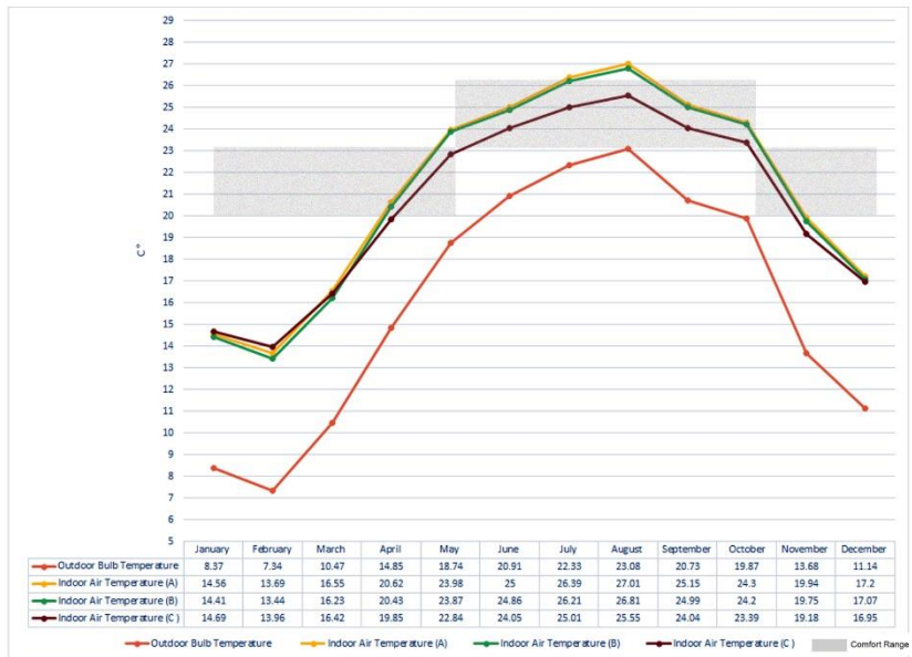
Figure 63: East vs. West Envelope at Roof Level vs. East Envelope at Ground Floor Level
