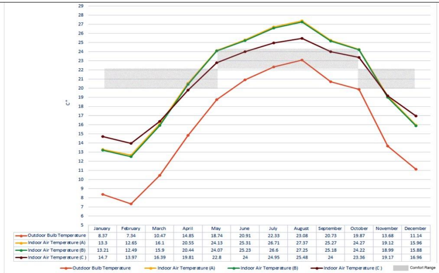
Figure 60: East vs. West Envelope at Roof Level vs. East Envelope at Ground Floor Level
