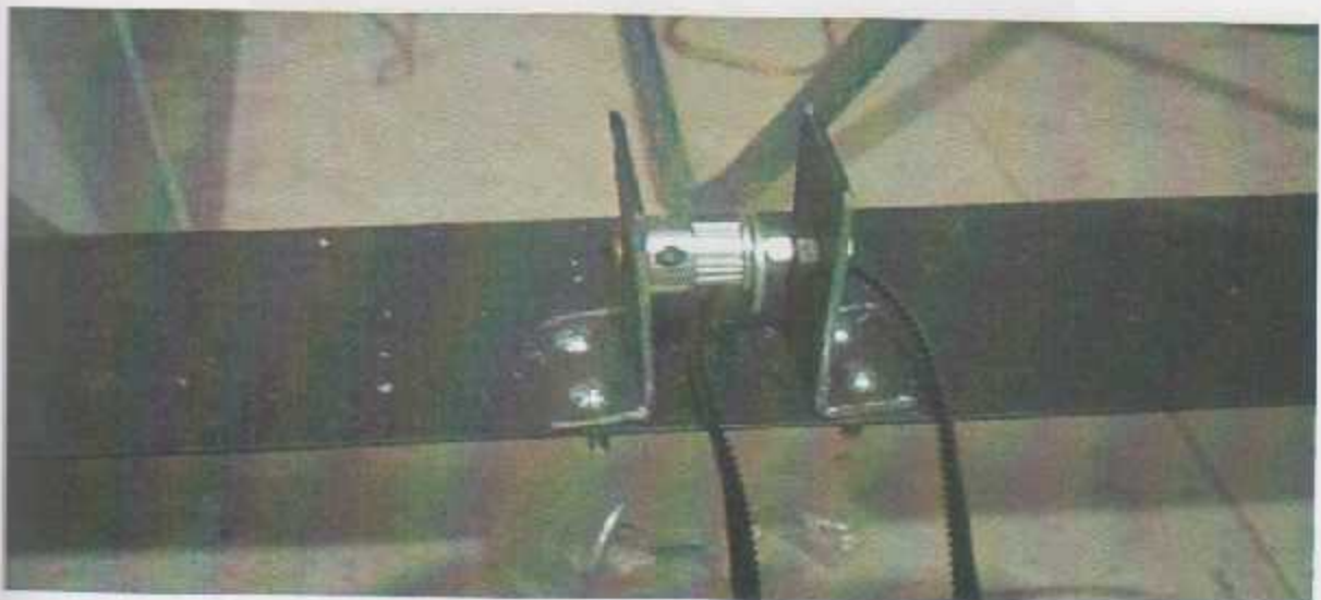
Figure 5.16: Timing Pulley installation
