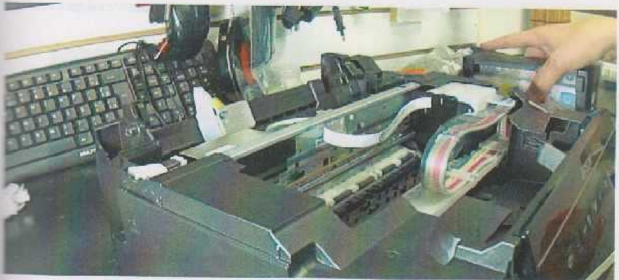
Figure 5.1: removing the scanner unite
