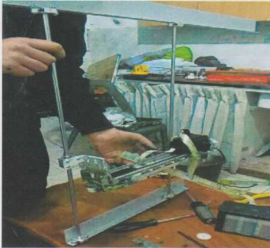
Figure 5.6: Linear guide motion and Y-axis installation
