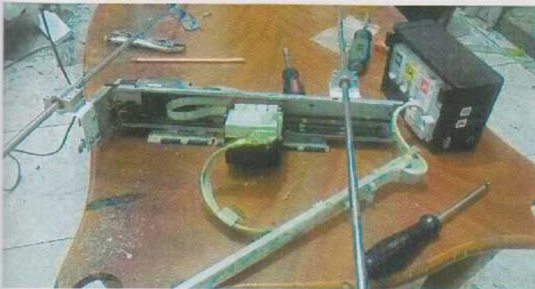
Figure 5.5: connect the bearing with printer head
