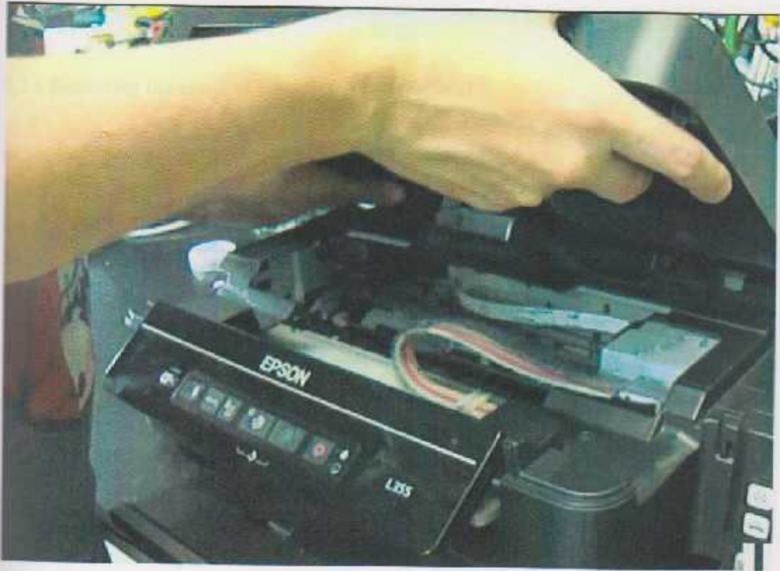
Figure 5.1: removing the scanner unite
