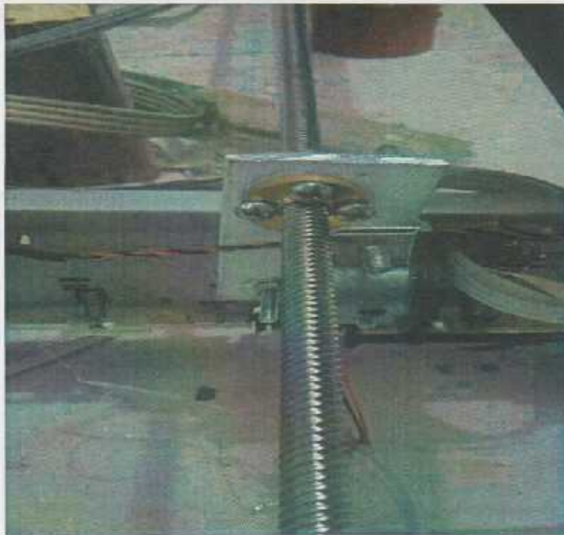
Figure 5.11: Screw nut installation
