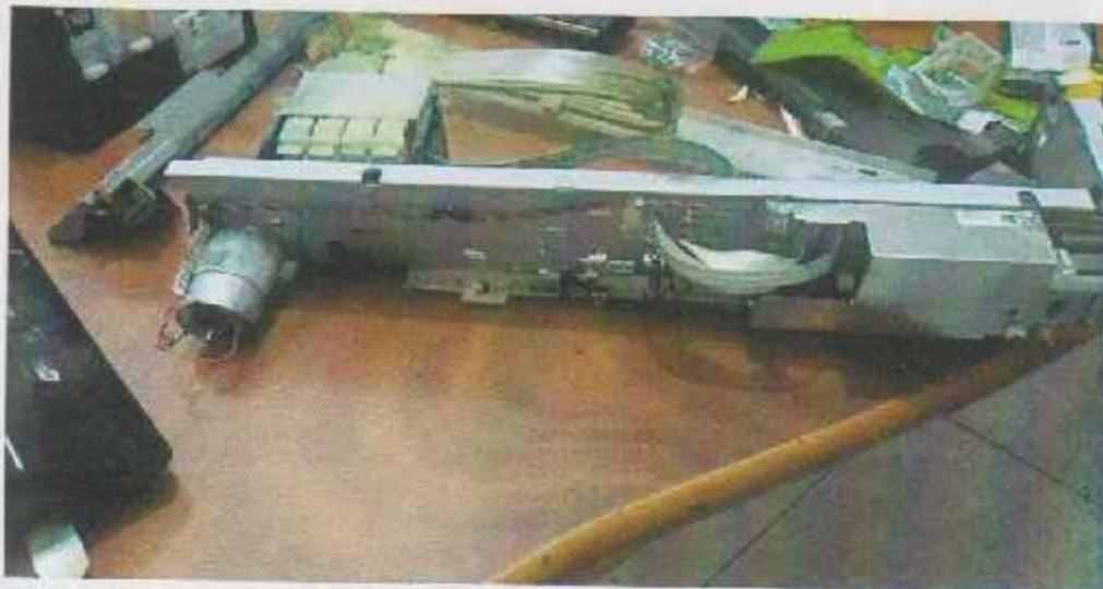
Figure 5.4: extraction the printer head
