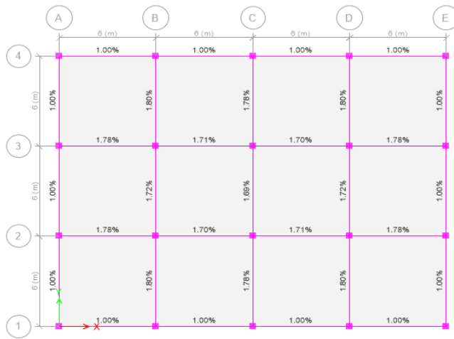
Figure 7.15 Output Design of the 6-Story Structural Building Showing the Required Reinforcement Area (mm) with Beam A (40cmX55cm), Beam B (30cmX50cm).
