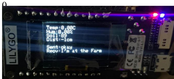
(a) Transmitter: Sending commands and data.
