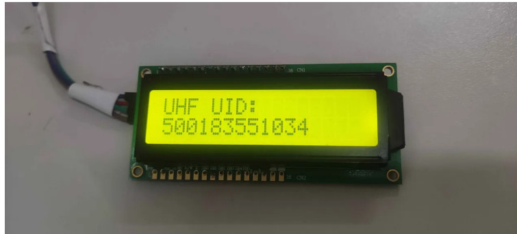
Figure 5.5: Reading Tag ID using VM5GA Module and Displaying it on LCD.
