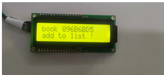
Figure 5.4: Reading Tag ID using RC522 Module and Displaying it on LCD.
