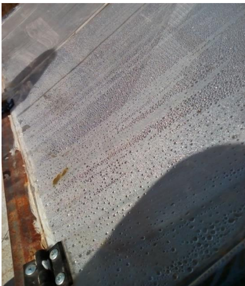
Figure 6.5: Condensation of water on the surface of the inner cover of the system
