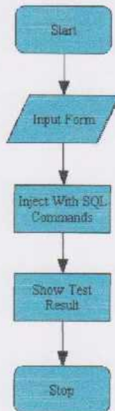
Figure 4.16: SQL Injection Test Flowchart
