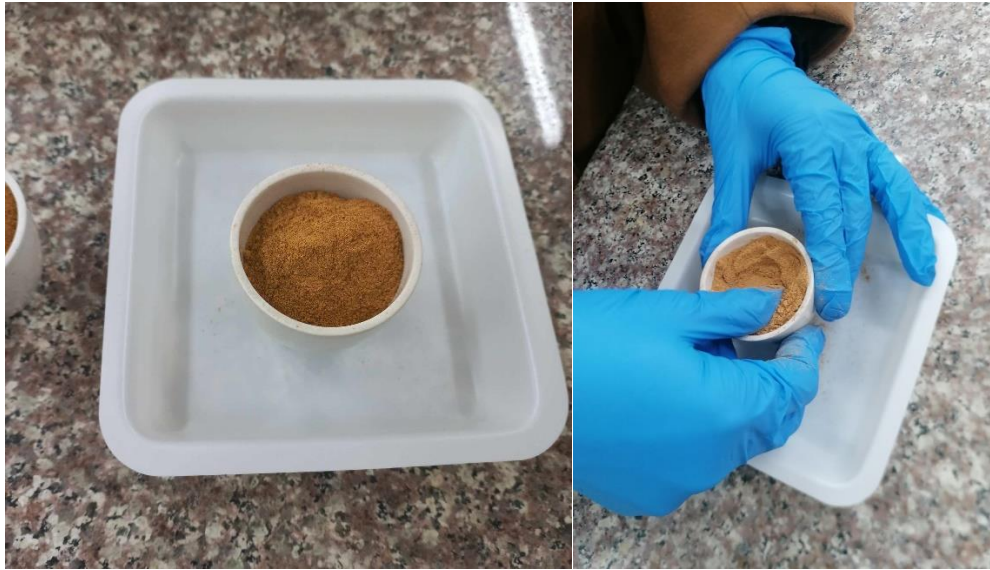
Figure A.5: packing to crucible.
