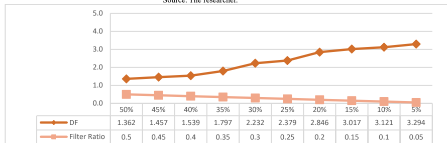
Fig. B.55. day light factor and filtration ratio achieved for ordinary window when WFR 5%/North. . Source: The researcher.
