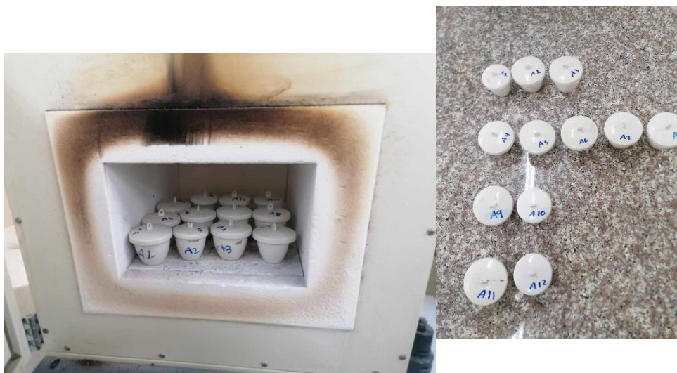
Figure A.6: The crucible put at muffle furnace.
