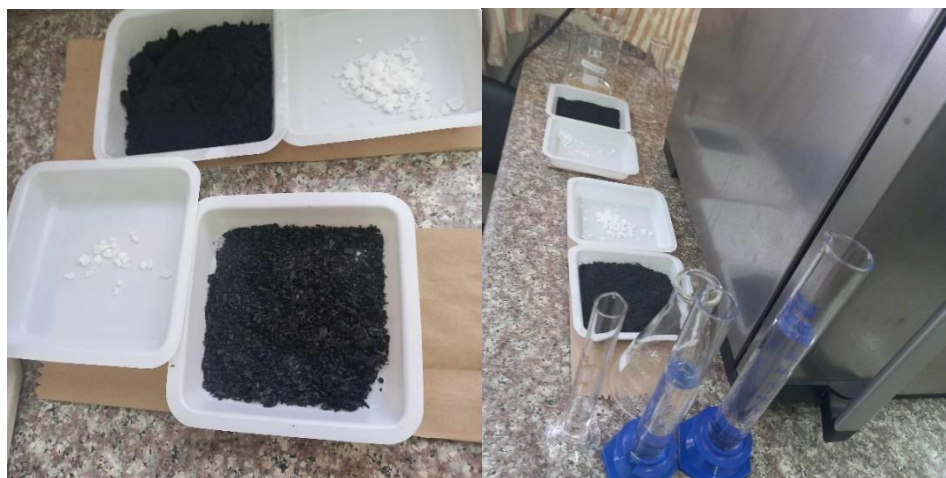
Figure A.7: biomass, distilled water and impregnation reagent.
