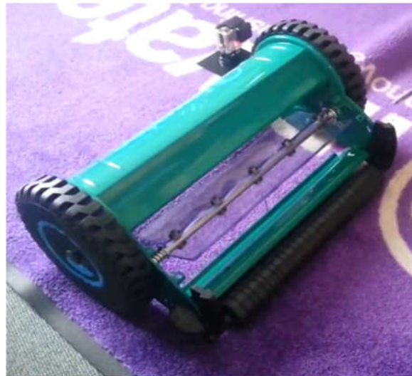
Figure 1.17: Collecting mechanism with metal blades
