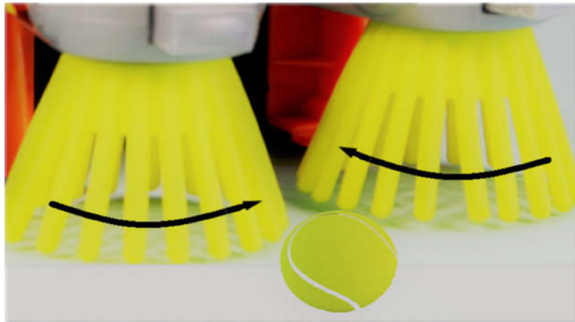
Figure 1.7: Collecting using two cylinders with vertical actuators
