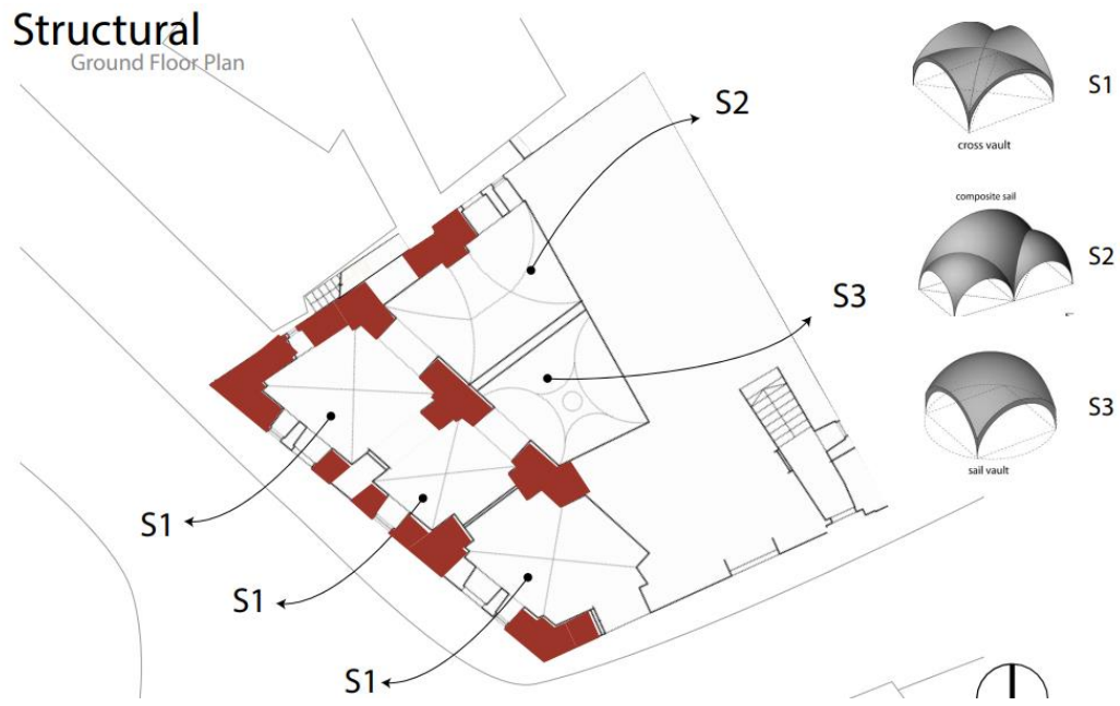
Figure 3.3: structural system for zaitoun building.
