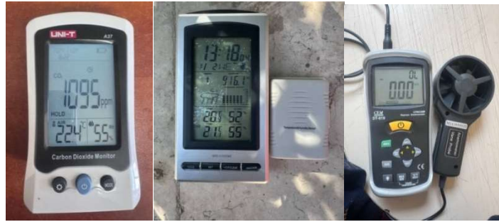
Figure 3-11 calibration tools(a- UNI-T A37 Digital Carbon Dioxide, b- wireless weather station ,c- DT-619 CFM/CMM Thermo-Anemometer)
