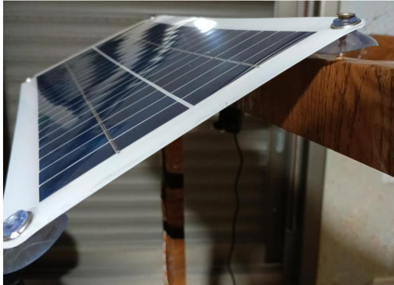
Figure 4.20 Solar panel at 45° angle
