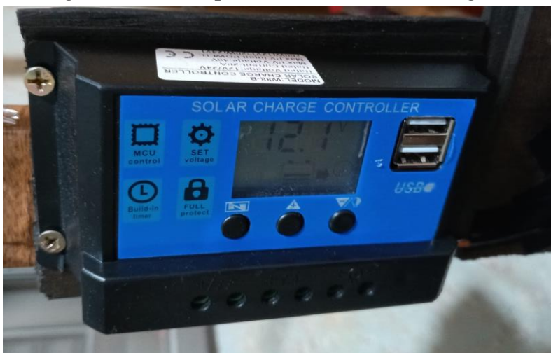
Figure 4.28 Solar charge controller testing
