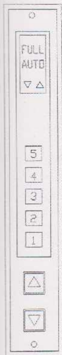
Fig 3.2 car operating panel
