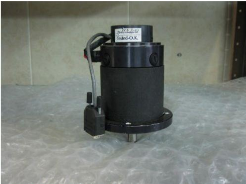
Fig.I: DC brushed servo motor
