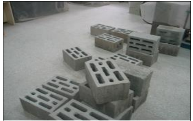
Figure 5. Recycled concrete block with three rows of holes. Zhu et al. [10]
