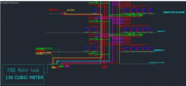
(b) Raiser Connection with Pumps
