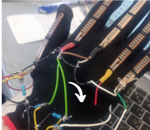
Figure 4.2: Loose In Wires Connection
