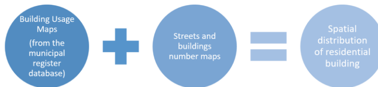
Figure 4.4: The procedure for mapping the distribution of dwellings begins with the municipal register database and a shape file of streets and building number maps.
