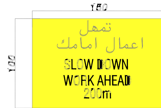
WORK AHEAD SIGN PROVIDED AT 500m AND 100m LEFT AND RIGHT
