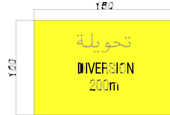
DIVERSION SIGN PROVIDED AT 500m AND 100m LEFT AND RIGHT
