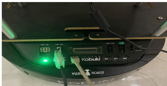
Figure 4.2: Connect Kinect sensor to Turtlebot.
