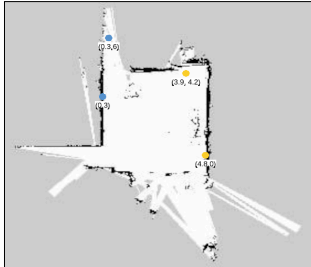
Figure 5.12: Defects localization results.
