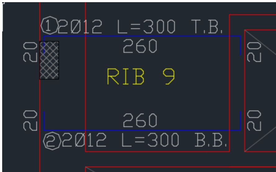
Figure 26: Reinforcement of Rib 9 in Building
