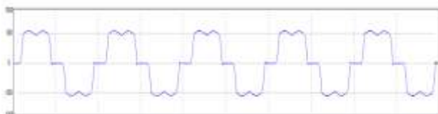
Fig. 7: Selected three-phase AC-DC converter with its distorted current.
