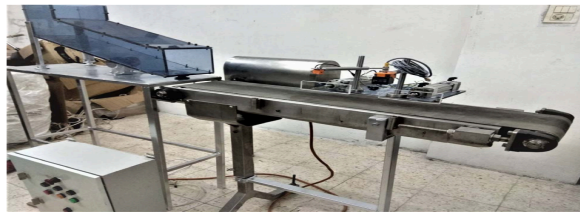
Figure 2.4: Automatic Sorting Machine. [8]
