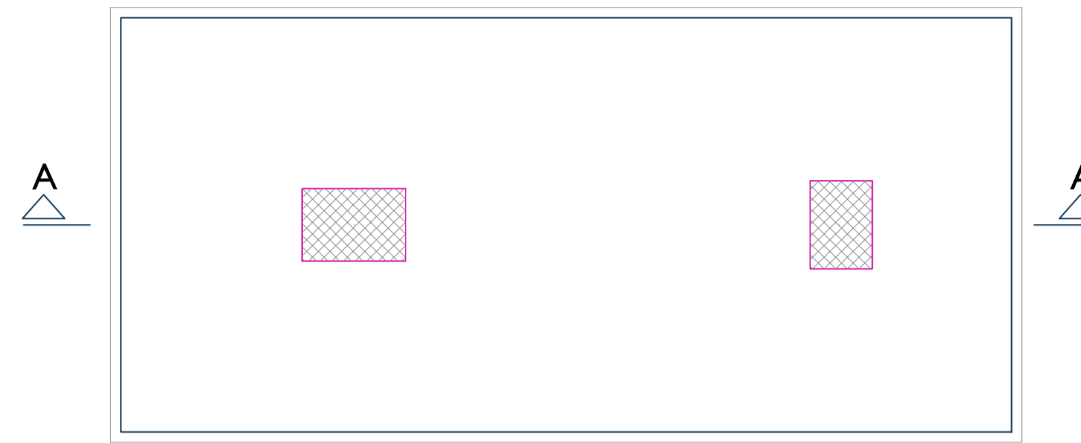
Continuous Footing 3 CF3(8.60x4.00x1.00)
