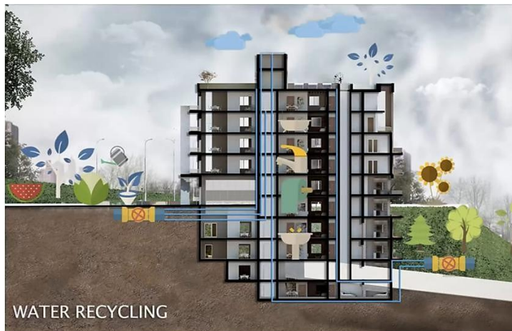
Fig. 4. 8: Gray water recycling system (SHTAYYA, 2018)
