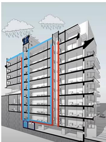
Fig. 4. 7: Rain water collection system (SHTAYYA, 2018)
