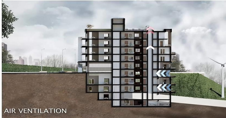
Fig. 4. 11: Air cross-ventilation through the building (SHTAYYA, 2018)
