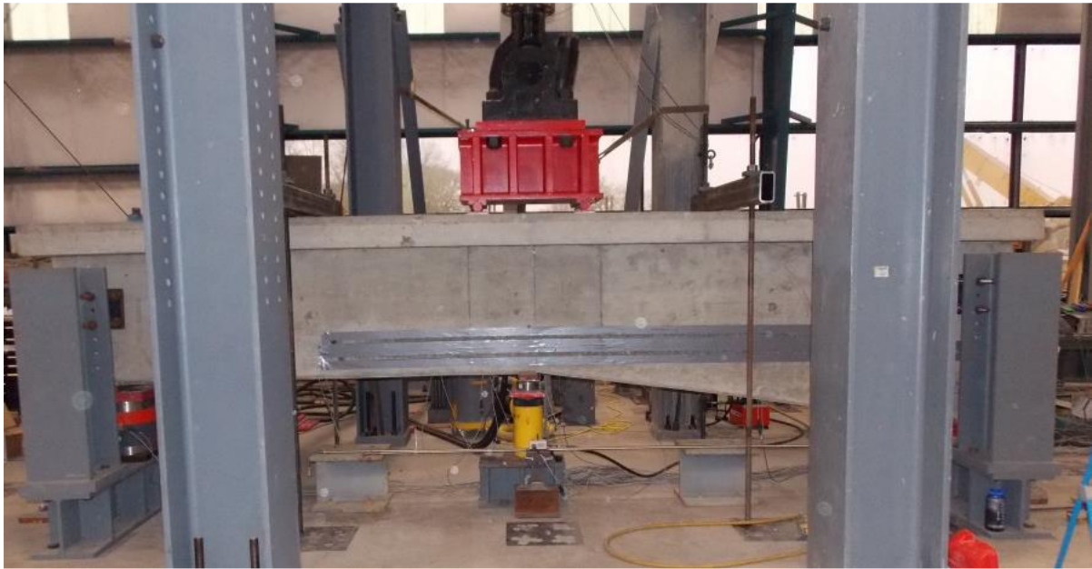
Figure 16: View of flexural specimen in Experimental test setup (Higgins et al., 2017)
