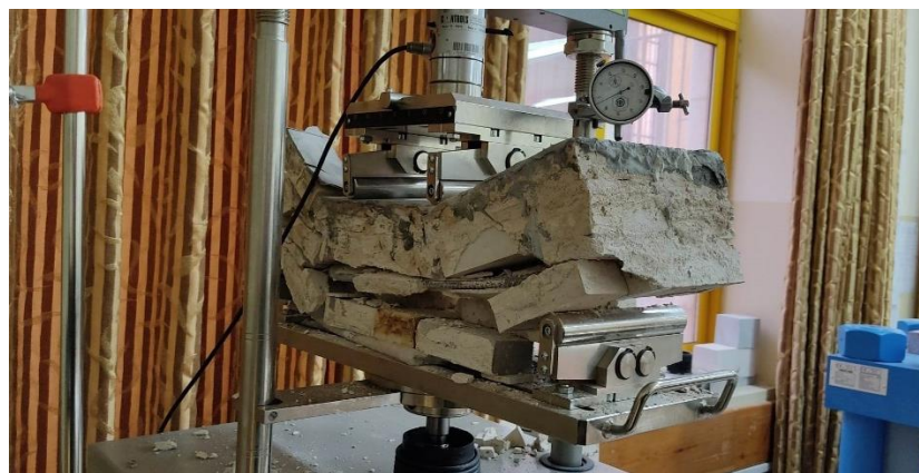
Figure 4.31: Flexural Strength sample of 55*15*10cm double leaf beam with 2 steel bar \phi 6. Source: researcher
