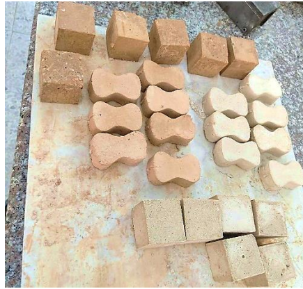
Figure 4.6: Compressive and Tensile samples of lime mortar and lime mixtures. Source: researcher
