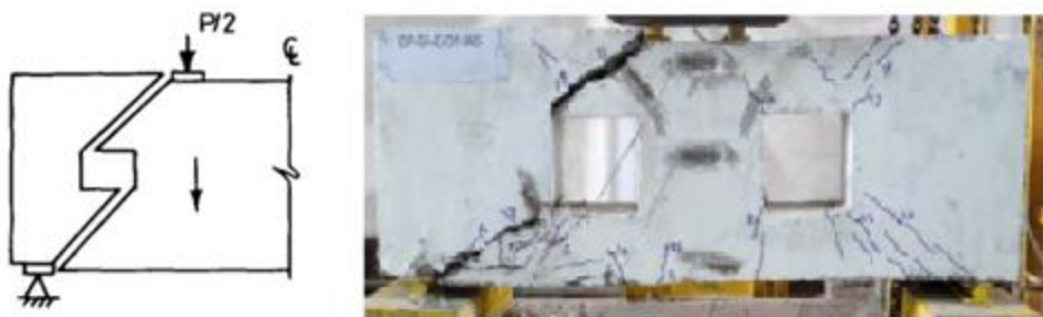
Figure 7: mode B failure, failure of deep beams left [Mansur and Alwis, 1984], right [jasim et al 2020]
