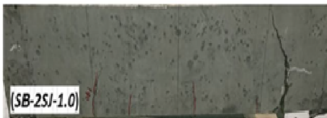
Figure 25: failure mode (tension damage ) of experimental and FE with UHPC.
