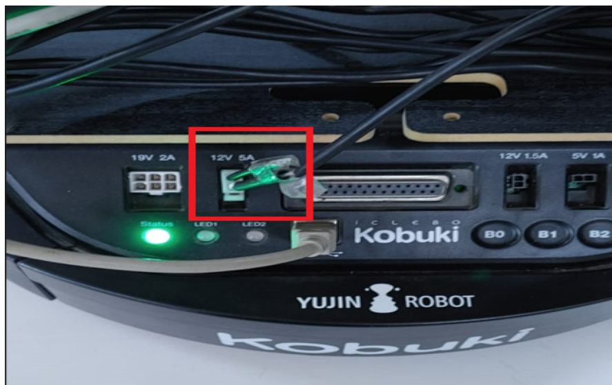
Figure 4.2: Connect XBOX 360 Kinect Sensor to Kobuki
