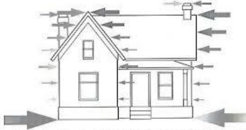
Horizontal earthquake forces (back-and-forth shaking) create 'whipping' forces in all parts of a building. These forces must transfer between parts of the building to the foundation.
