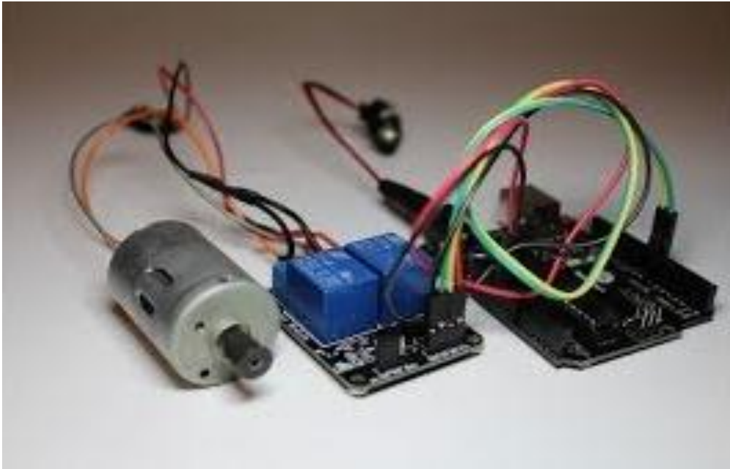
Figure 5.4: Connections Between ESP32 and DC motor
