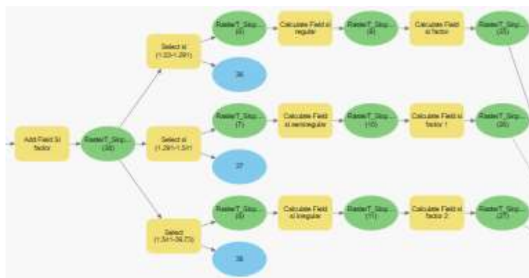
Figure 5.12 model builder to classify lands depending on the shape index and calculate the factor to this category
