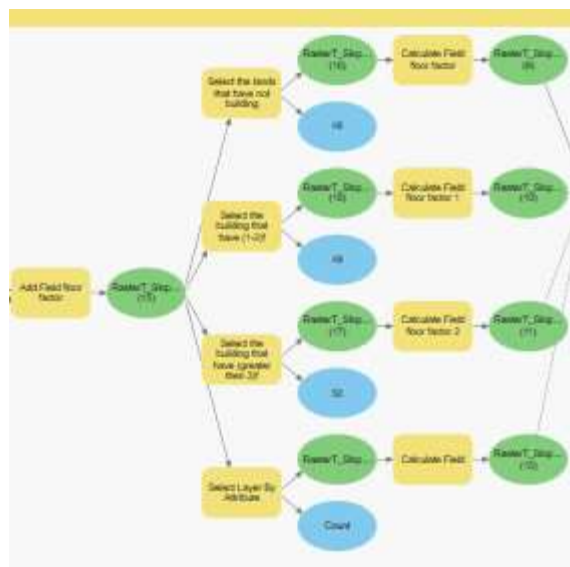
Figure 5. 16 model builder to calculate the factor of lands depending on number of floors
