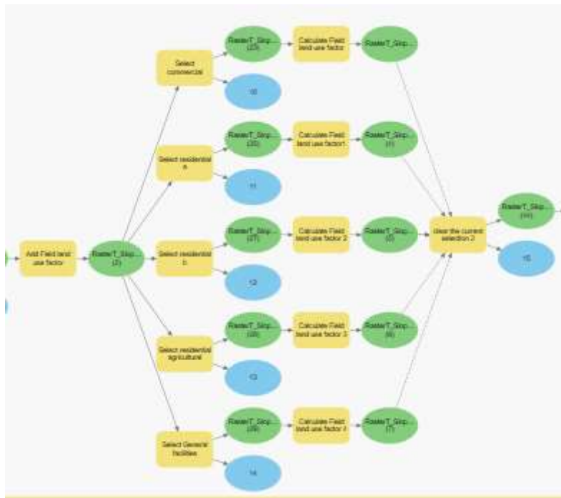
Figure 5. 6 model builder to calculate factor for each land use classification
