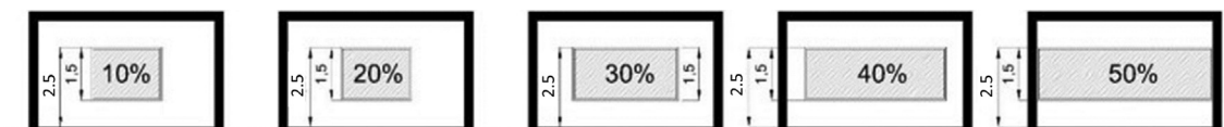
Fig. 7. Simulation cases of the studied room with the change of window wall ratio.
