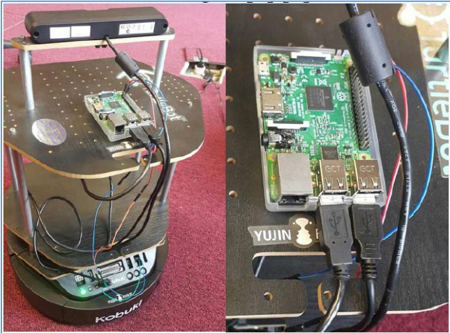
Figure 1.9: Turtlebot mobile robot used raspberry pi as the main processing unit.[11]
