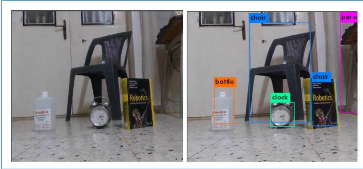
Figure 5.1: An input image (left) is applied to the YOLO algorithm and an output image (right) with each detected object.
