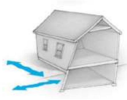
Figure(3- 5):Seismic Loads
