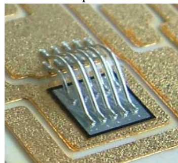
Fig. 5: One-sided LTJT with wire bonds
