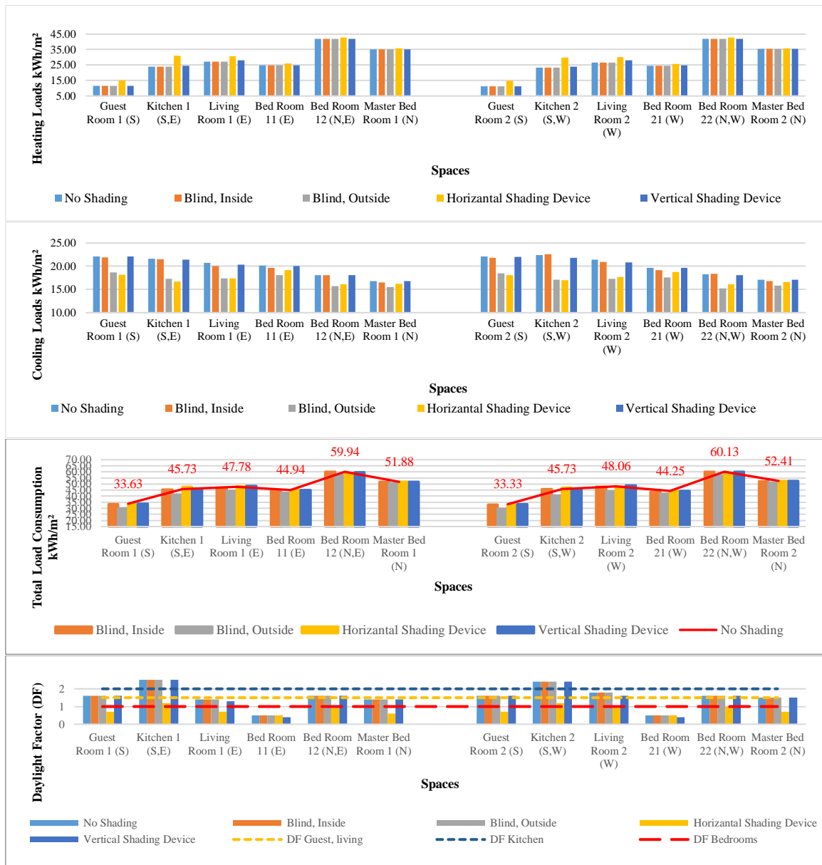
Figure 6.77: The effect of adding different types of internal and external shading devices, First floor, South oriented street.
