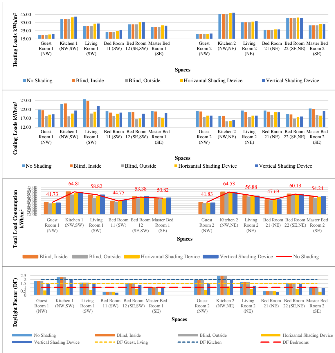
Figure 6.89: The effect of adding different types of internal and external shading devices, First floor, North-West oriented street.
