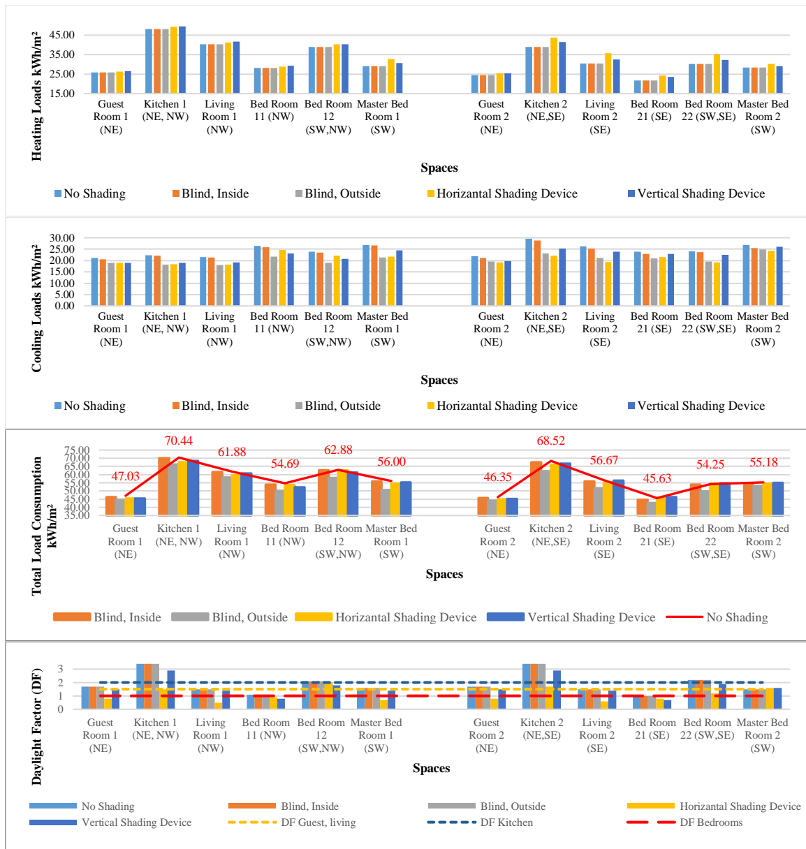
Figure 6.67: The effect of adding different types of internal and external shading devices, Third floor, North-East oriented street.
