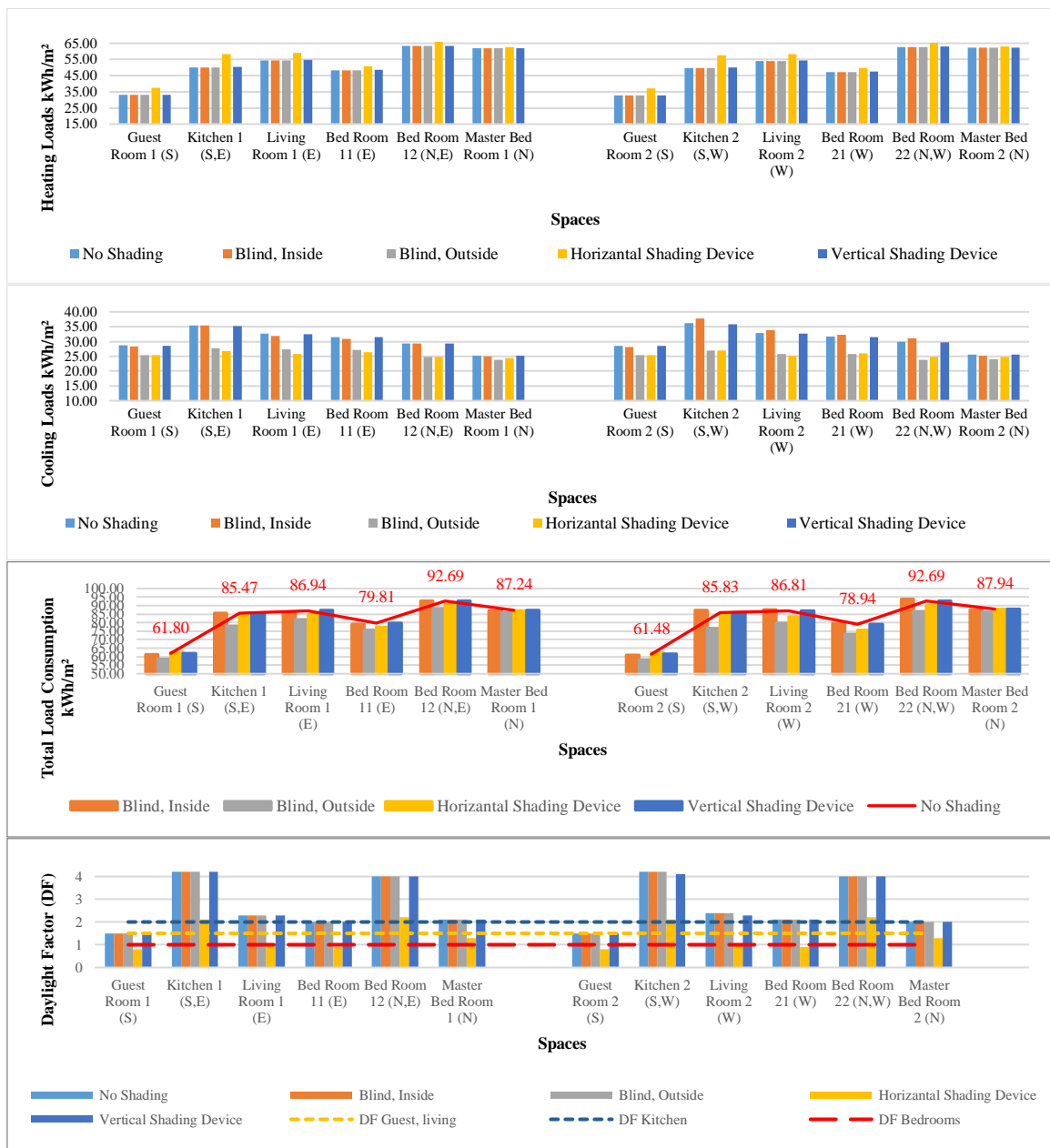
Figure 6.80: The effect of adding different types of internal and external shading devices, Fourth floor, South oriented street
