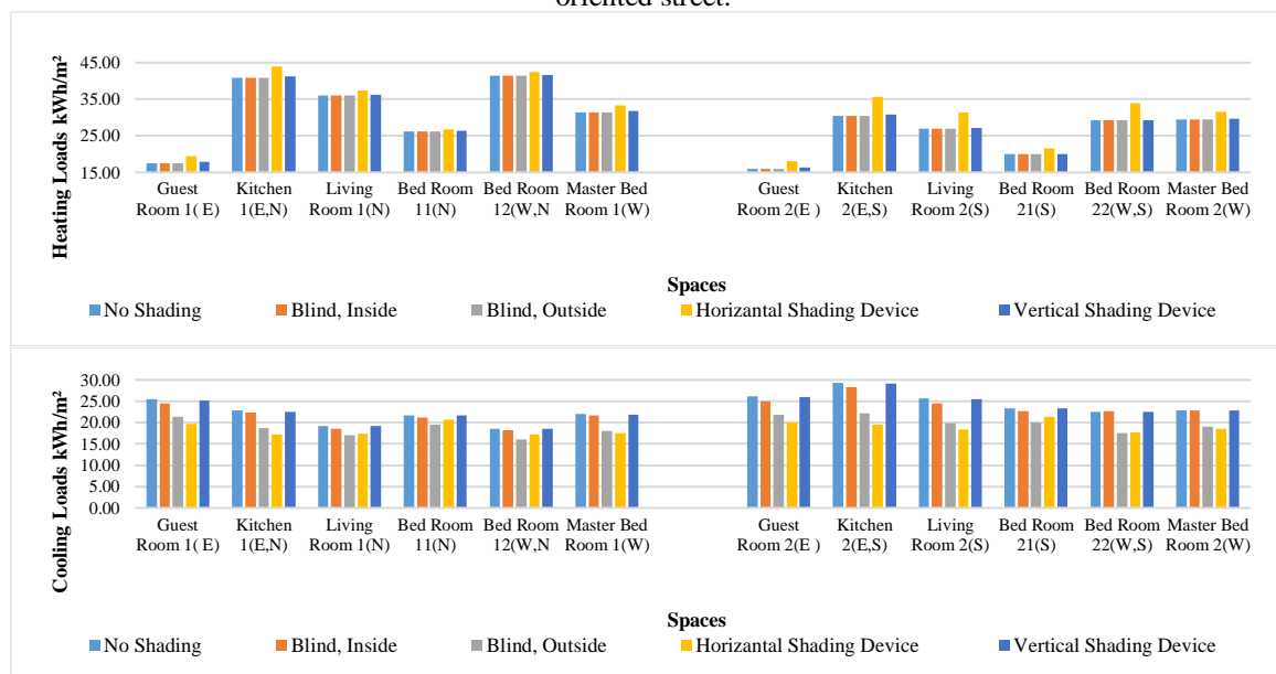
Figure 6.69: The effect of adding different types of internal and external shading devices, First floor, East oriented street.
