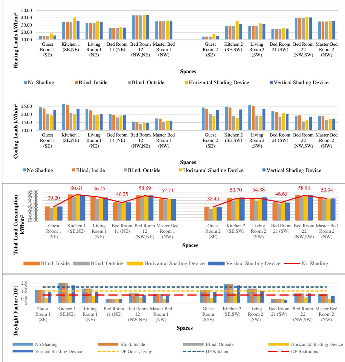
Figure 6.73: The effect of adding different types of internal and external shading devices, First floor, South-East oriented street.
