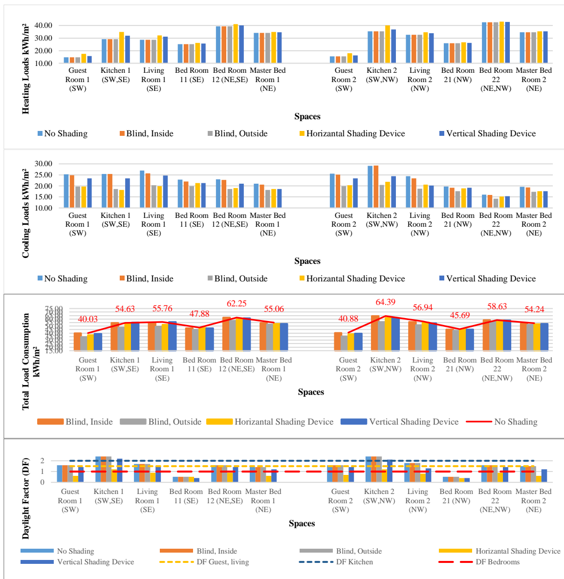
Figure 6.81: The effect of adding different types of internal and external shading devices, First floor, South-West oriented street.
