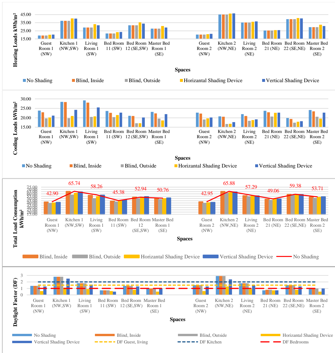
Figure 6.90: The effect of adding different types of internal and external shading devices, Second floor, North-West oriented street.
