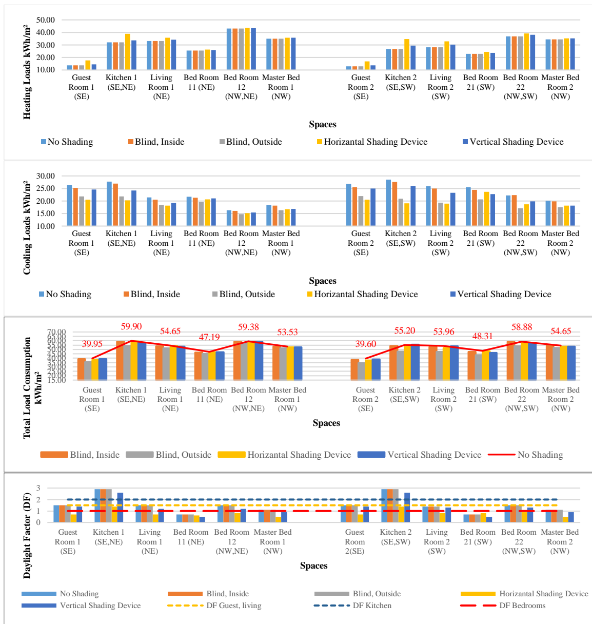
Figure 6.74: The effect of adding different types of internal and external shading devices, Second floor, South-East oriented street.
