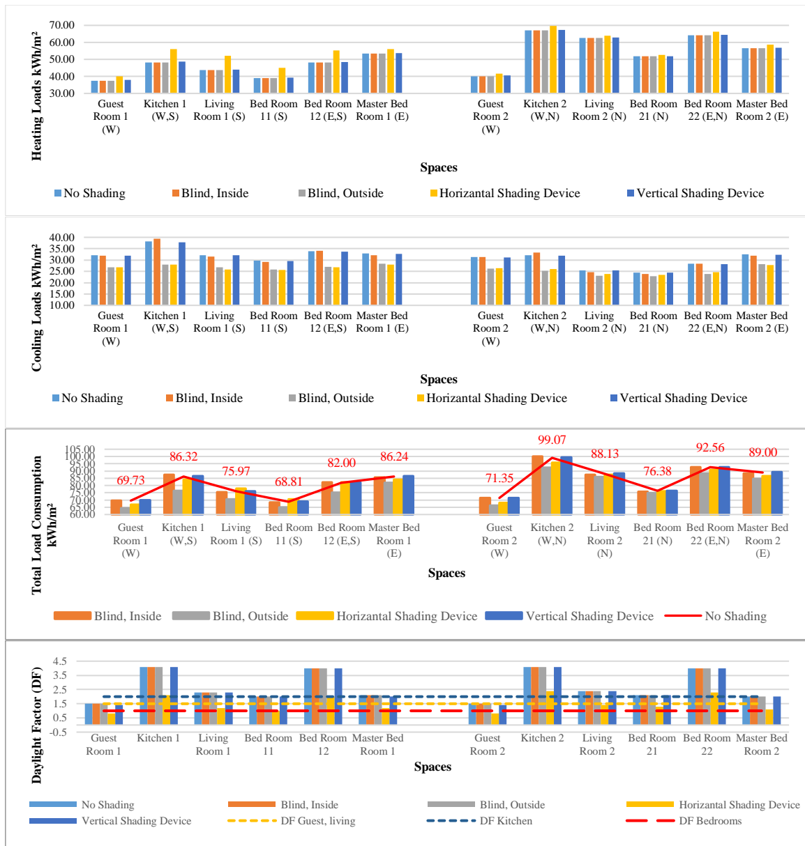
Figure 6.88: The effect of adding different types of internal and external shading devices, Fourth floor, West oriented street.
