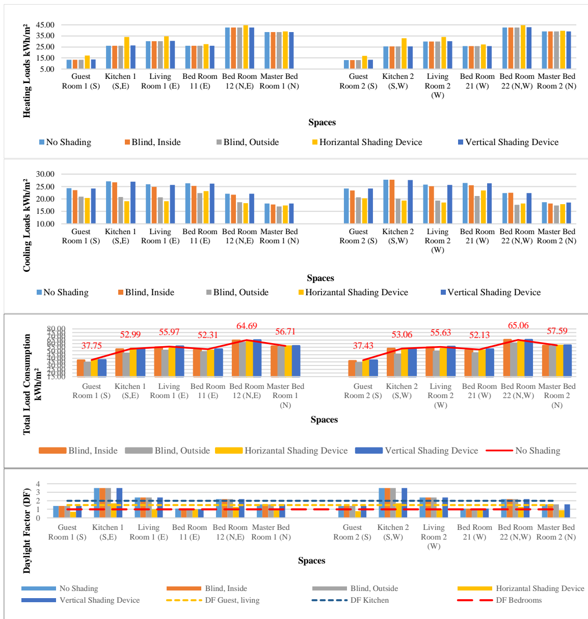
Figure 6.79: The effect of adding different types of internal and external shading devices, Third floor, South oriented street.
