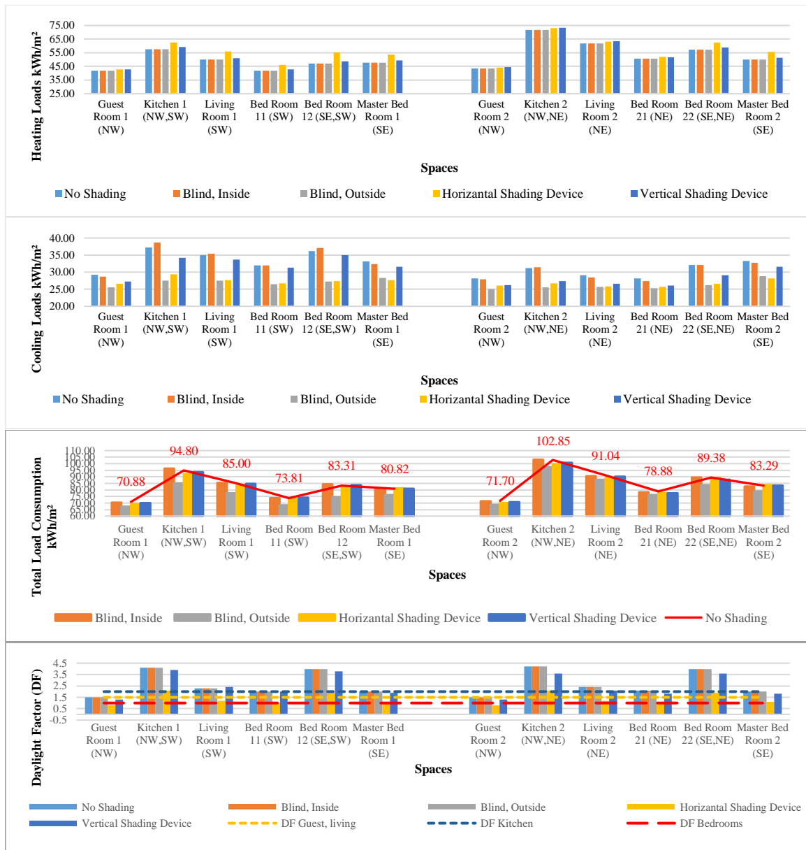
Figure 6.92: The effect of adding different types of internal and external shading devices, Fourth floor, North-West oriented street.
