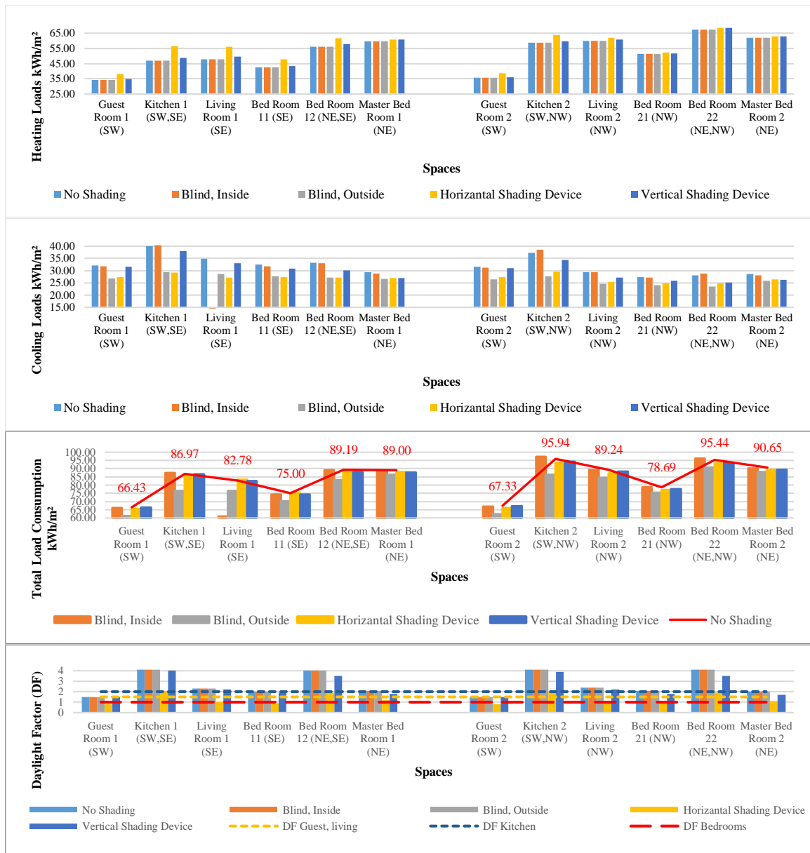
Figure 6.84: The effect of adding different types of internal and external shading devices, Fourth floor, South-West oriented street.
