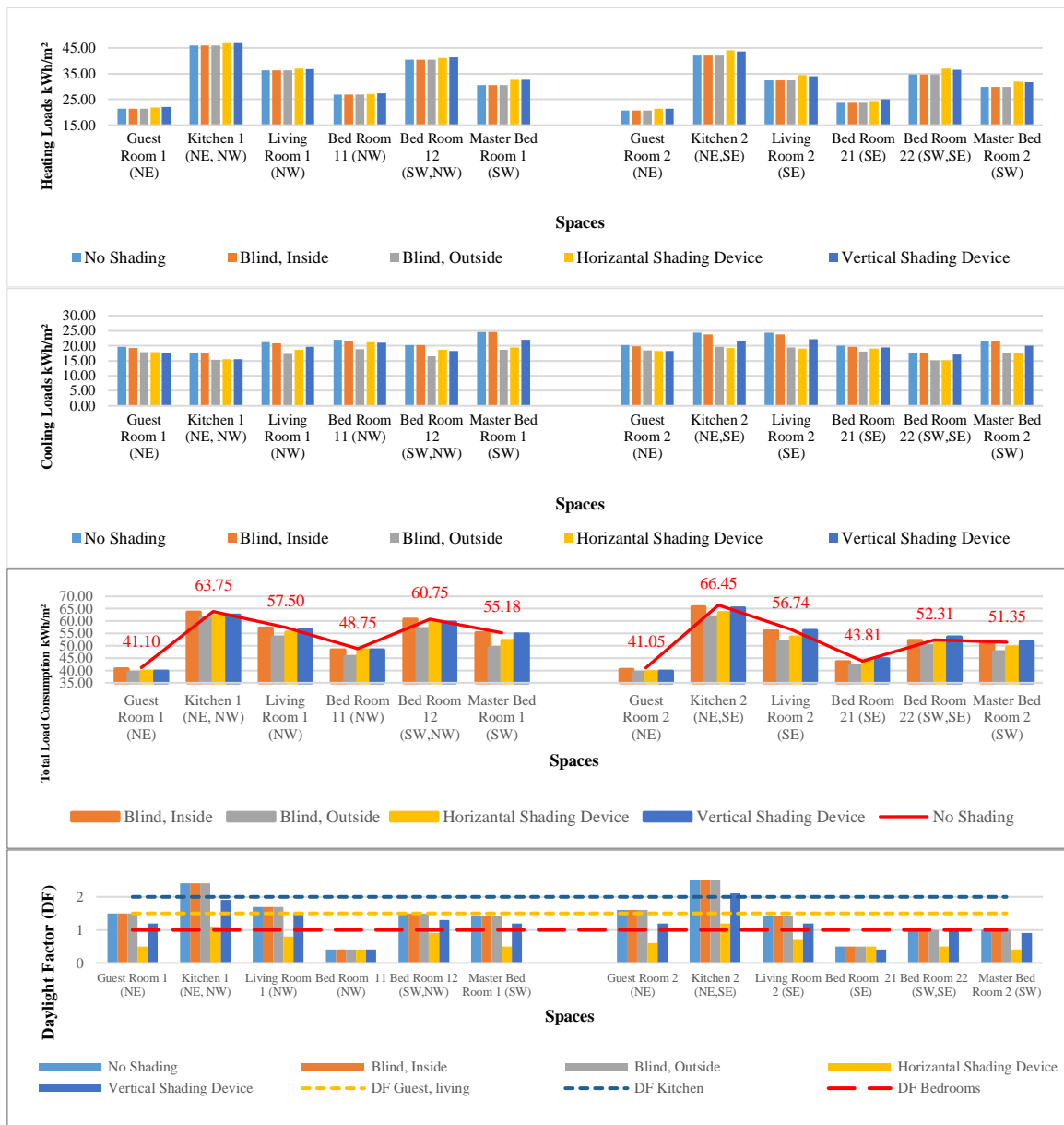
Figure 6.65: The effect of adding different types of internal and external shading devices, First floor, North-East oriented street.
