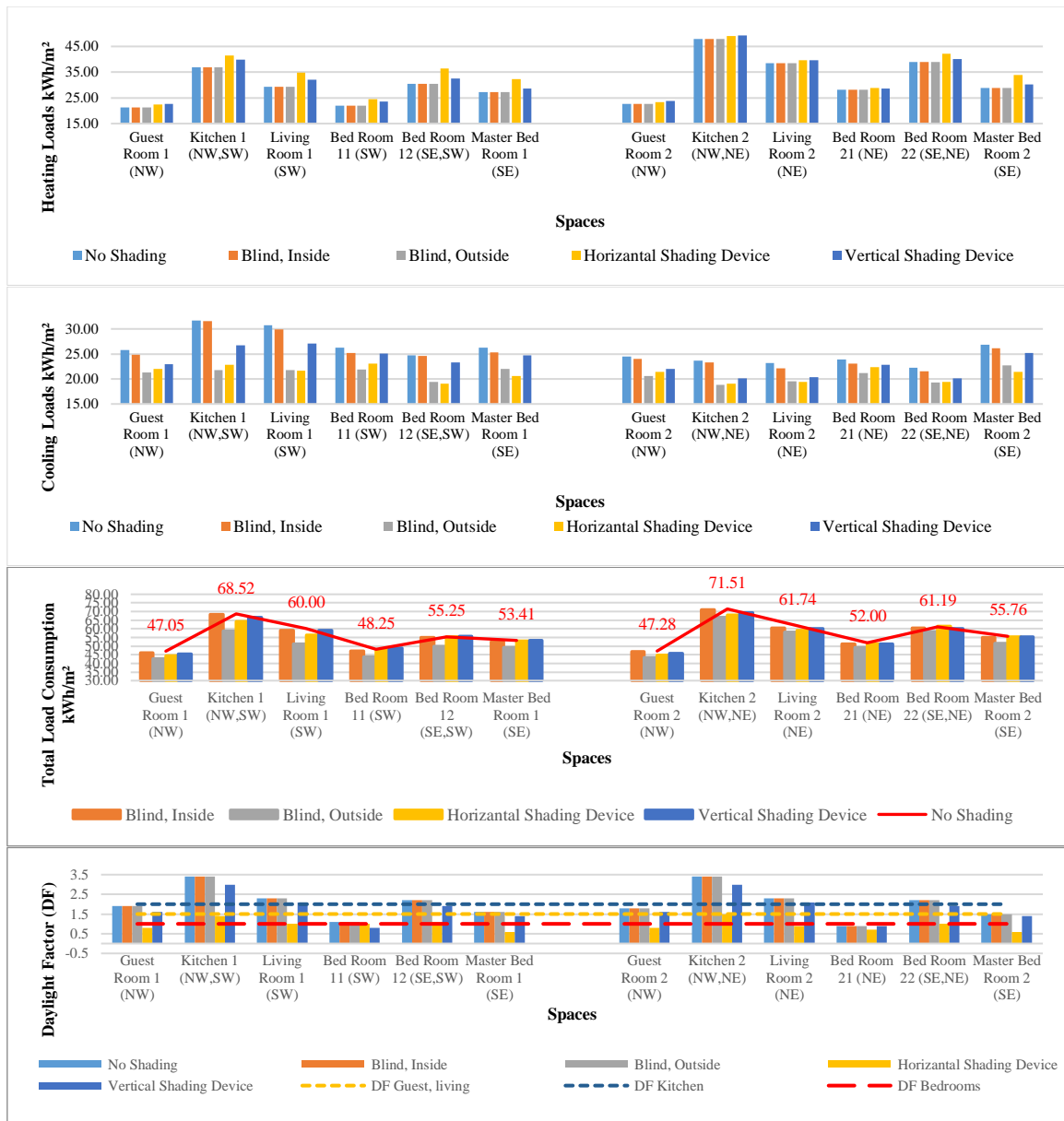
Figure 6.91: The effect of adding different types of internal and external shading devices, Third floor, North-West oriented street.
