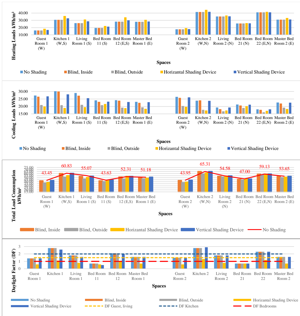
Figure 6.86: The effect of adding different types of internal and external shading devices, Second floor, West oriented street.
