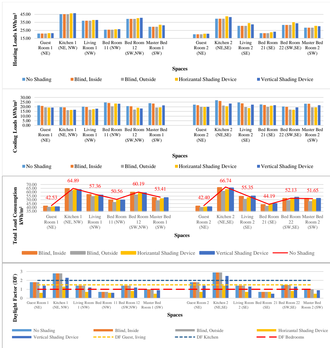
Figure 6.66: The effect of adding different types of internal and external shading devices, Second floor, North-East oriented street.
