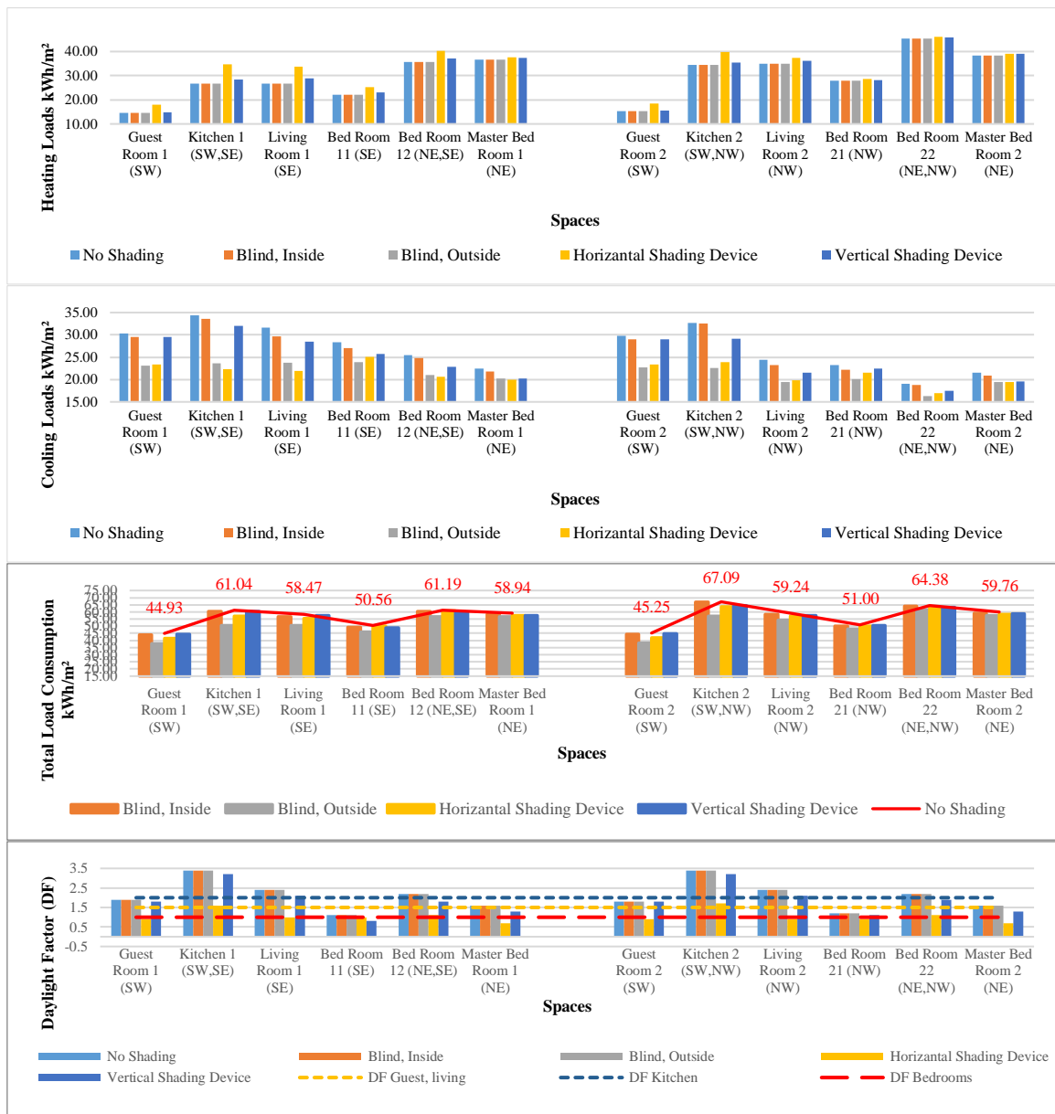
Figure 6.83: The effect of adding different types of internal and external shading devices, Third floor, South-West oriented street.
