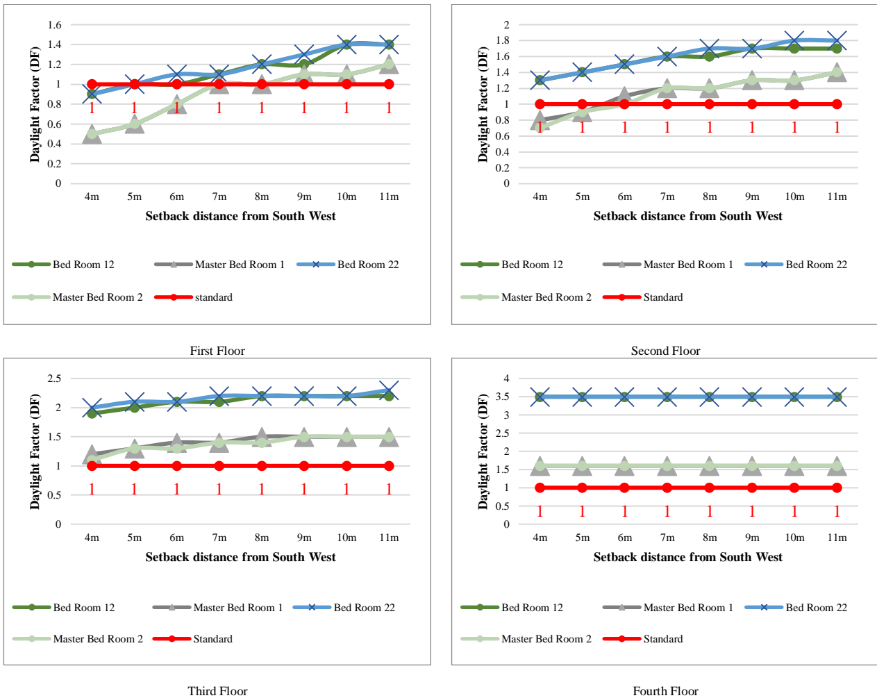
Figure 6.15: North-East Street oriented street case Daylight Factor results when South-West setback was increased.
