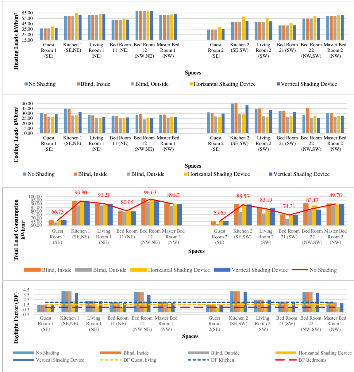
Figure 6.76: The effect of adding different types of internal and external shading devices, Fourth floor, South-East oriented street.
