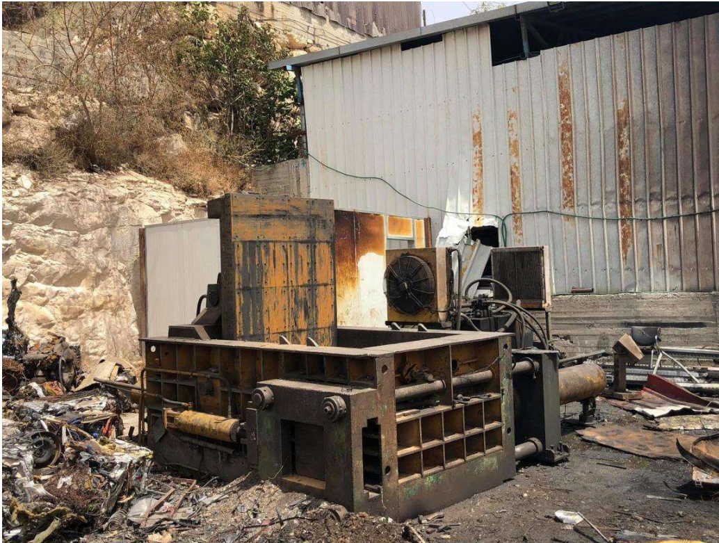
Figure 5.1:Scrap Metal Crusher Machine after installation
