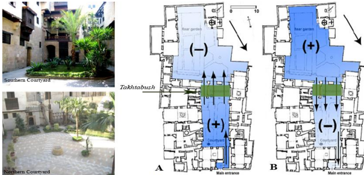
Figure 2.6: The passive cooling system of The Takhtabush, Al-Suhaymi house, Egypt, where (A) the air movement during noon, and (B) the air movement afternoon, edited from (Attia,2006, p.2,).
