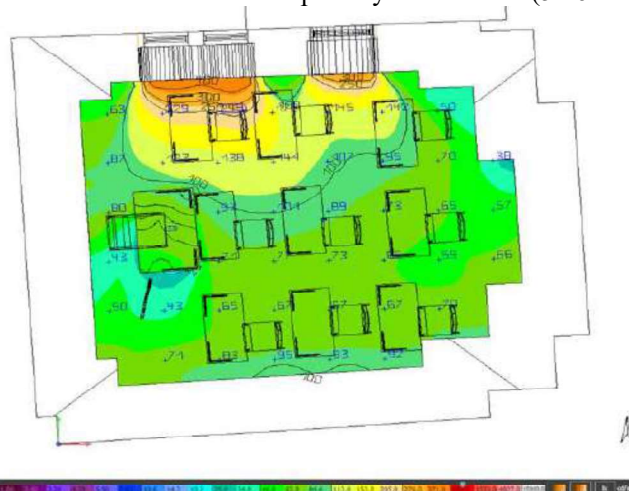
Figure 7: Contour diagram for classroom"2" optimization by adding Ground area: 22.85 m 2 | Reflection factors: Ceiling: 75.8 %, Walls: 75.8 %, Floor: 60.8 % | Maintenance factor: 0.80 (fixed) | Clearance height: 2.381 m - 3.100 m | work plan height:0.6cm.
