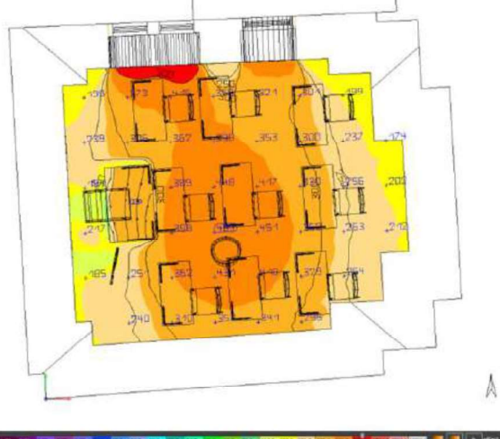
Figure 9: Contour diagram for classroom “2” optimization by adding pipe light (93.8lux to 304 lux)
