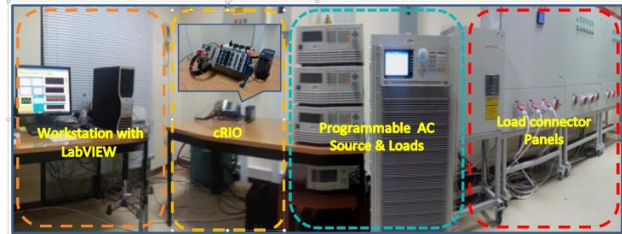
Fig. 4. The experimental setup in a power quality laboratory.
