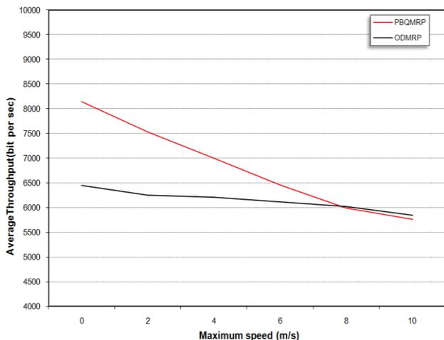
Figure 2. Average throughput vs. node mobility speed.
