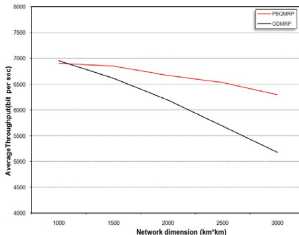
Figure 3. Average throughput vs. network size.
