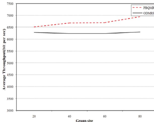
Figure 4. Average throughput vs. multicast group size.
