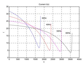
Figure 9. Simulation results of the motor current at various frequencies  $I_{ph} = f(n)$ .
