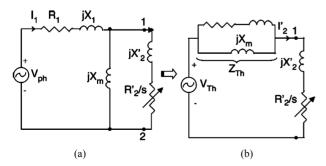
Figure 6. Equivalent circuit of 3-phase induction motor. (a) Equivalent circuit for one phase; (b) Application of Thevenin's theorem.
