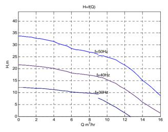
Figure 8. Simulation results of the pump performance H = f(Q).
