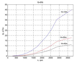
Figure 10. Simulation results for pump performance at different heads (elevations).
