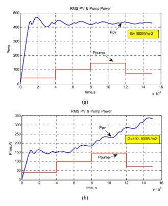
Figure 13. Generated and consumed power at various irradiations. (a) Power diagram at constant irradiation; (b) Power diagram at various irradiations.
