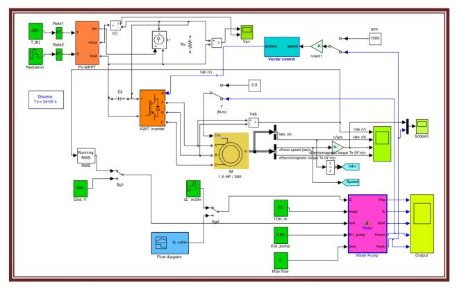
Figure 11. Matlab/Simulink model of induction-motor pump.
