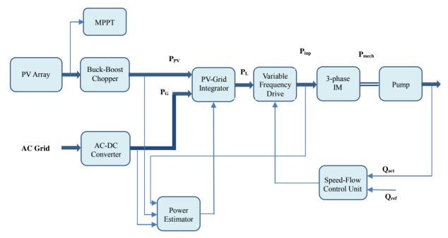
Figure 1. Functional block diagram of proposed model.
