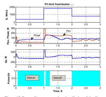
Figure 15. Power diagram at various irradiations & loading status.
