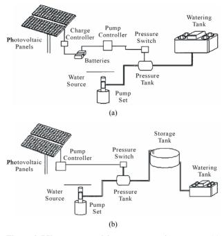
Figure 4. PV system energizing water-pumping systems. (a) Direct-coupled water-pumping systems; (b) Battery-coupled water-pumping systems.
