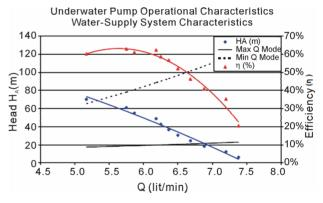
Figure 5. Water pump operational characteristic.
