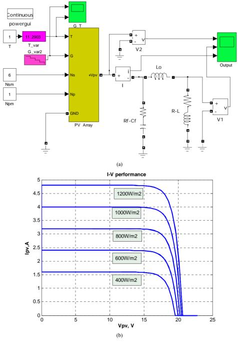
Figure 3. PV model with I-V performances. (a) Proposed model for PV array in Simulink environment; (b) I-V performance of PV module.
