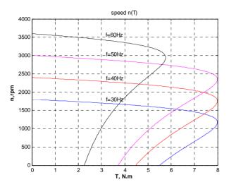
Figure 7. Simulation results of the mechanical performance of three-phase induction motor.
