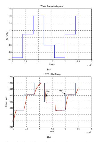
Figure 12. Simulation results of water flow-rate and obtained speed. (a) Water flow-rate diagram; (b) Pump actual & reference speed at 20 m elevation.
