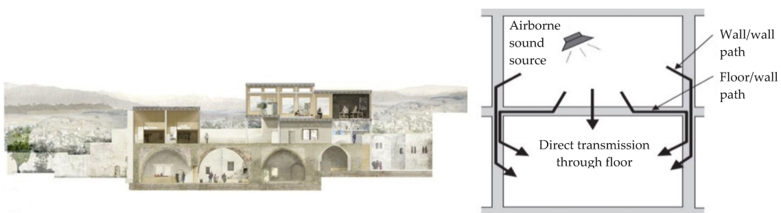
Figure 18. Comparison at the level of the internal noise transmission, low noise transmission through low rise buildings, Old (Left); high level of vertical noise transmission, New (Right).
