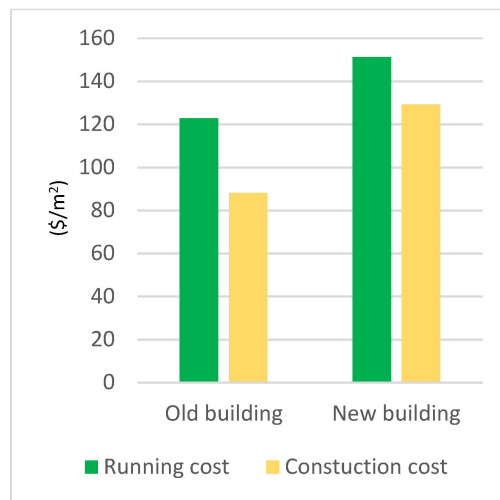
Figure 5. Comparison between the total cost of an old and a new building in Palestine. Adapted from [8].
