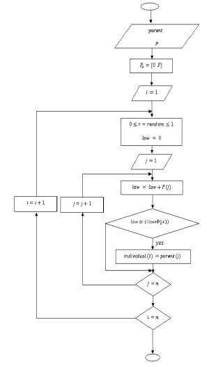
Fig. 9 Routlee wheel selection flow chart
