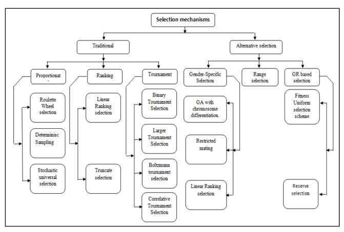
Fig. 1 Selection mechanisms
