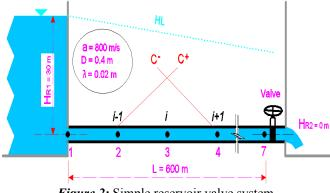
Figure 2: Simple reservoir valve system.
