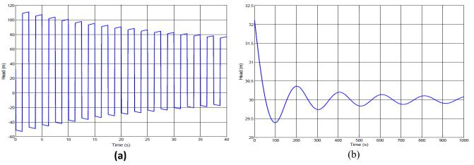
Figure 7: Transients in a pumping system (a) Head change versus time at the pomp and (b) Head change versus time at the pomp
