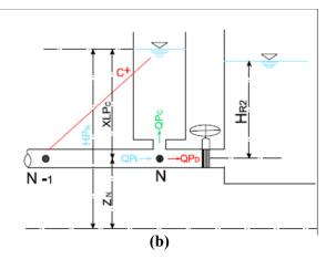
diameter of the pipe since the average velocity of flow is not excessive, the choice of material and class of pipe pressure to reduce pressure changes with a little risk of bursting or crushing, and finally the choice of valves whose closure durations are relatively slow.
