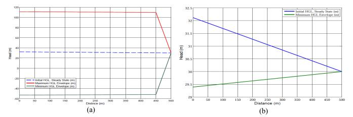
*Figure 8:* Hydraulic grade lines envelopes *(a)* Hydraulic Grade Lines (without Protection) And *(b)* Hydraulic Grade Lines (with Protection)
