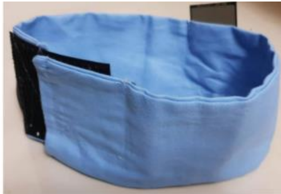
Fig 5.1 The strap contains Flexiforce sensor
