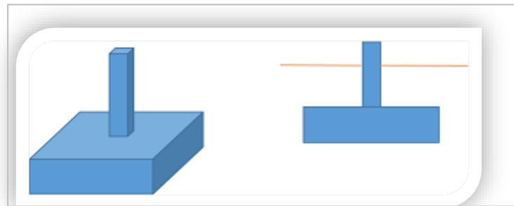
Picture 36: Isolated foundations
