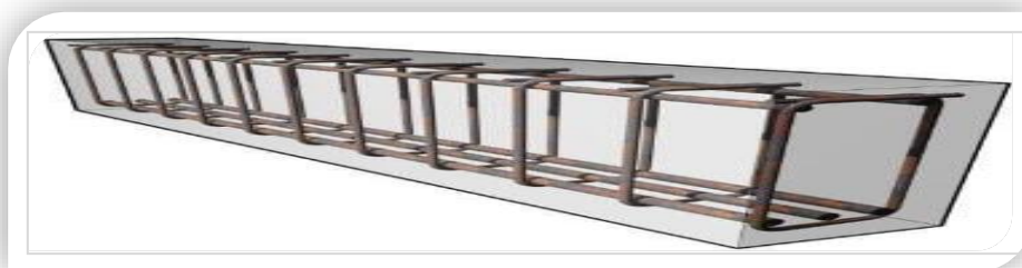
Picture 28: Reinforced concrete beam
