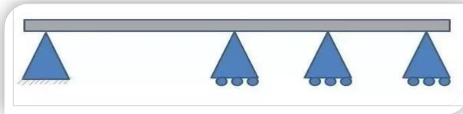
Picture 27: continuous beam
