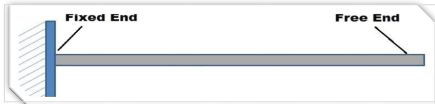
Picture 26: cantilever beam
