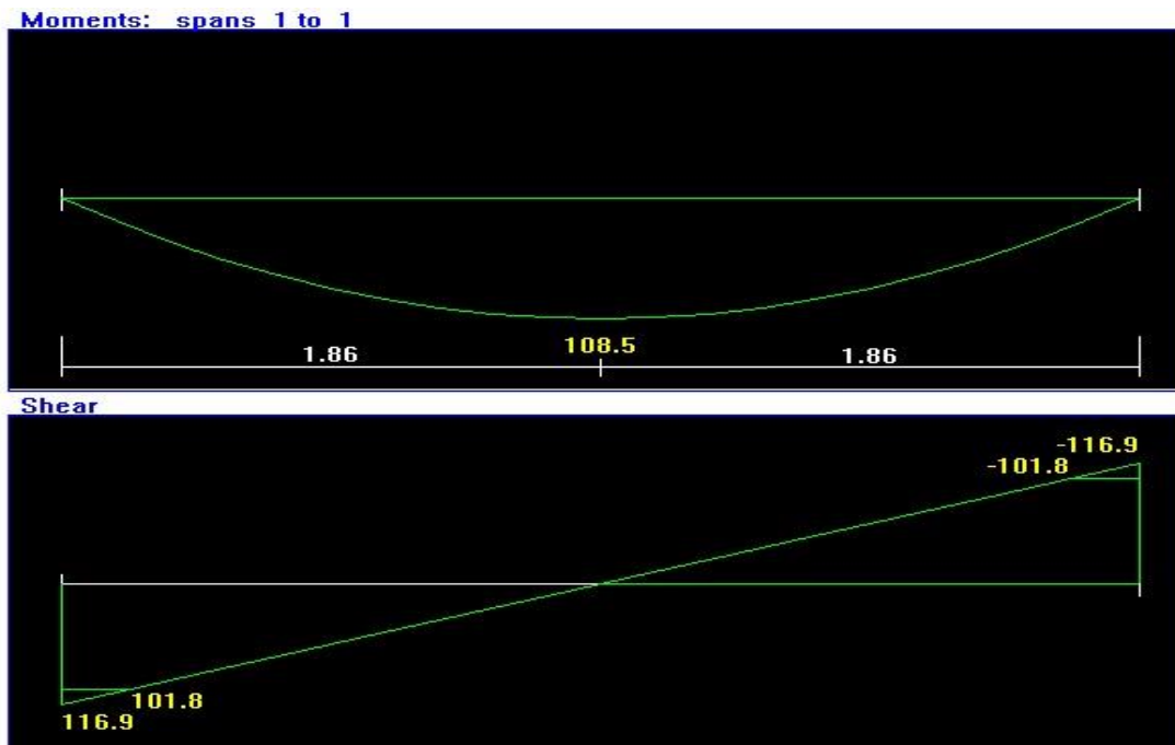
Figure 4. 11: Moment /Shear Envelope of basement wall
